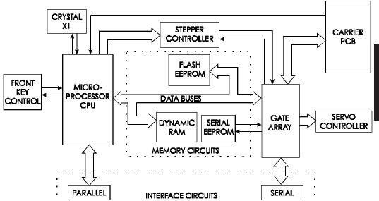
Figure 2-4. Main Printed Circuit Board.
